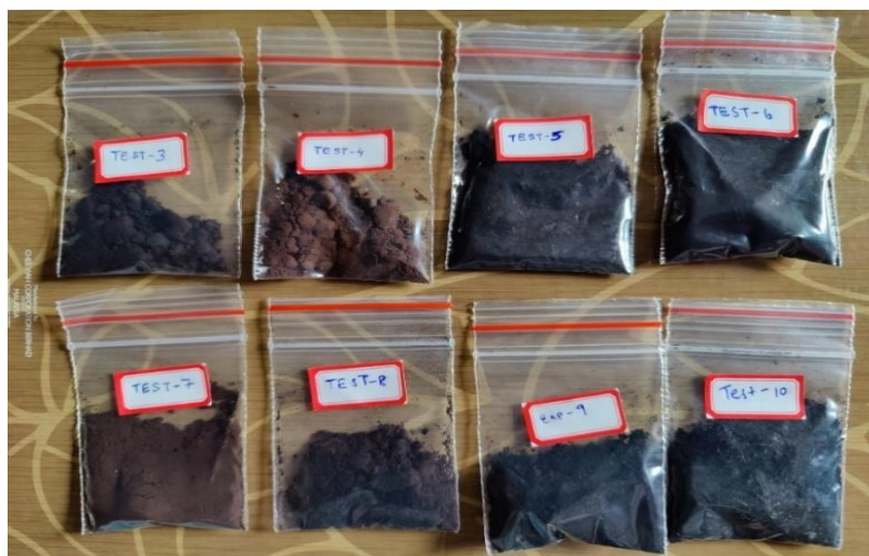
Figure 63: Partially or completely torrefied SCG from the designed solar torrefied.
