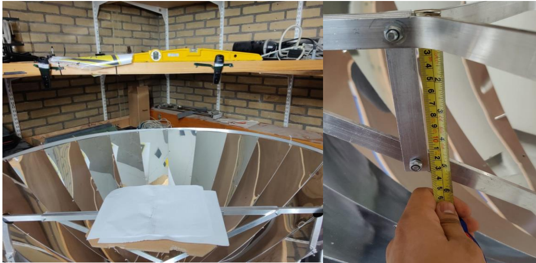
Figure 37: Arrangement of the 'EG Solar' cooker for the laser experiment to estimate the focal point.
