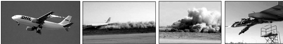
Figure 1 Emergency landing sequence using engines only and left wing structural damage due to SAM missile impact, DHL A300B4-203F, Baghdad, 2003
