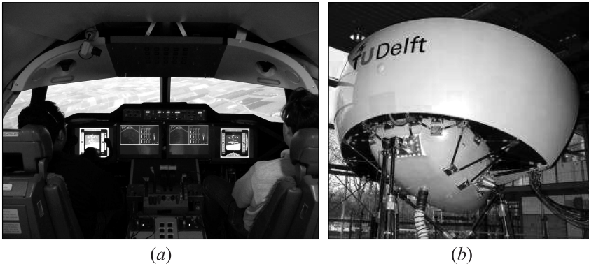
Figure 7 Evaluation of GARTEUR FM-AG(16) FTFC techniques in the Delft University SIMONA Research Simulator based on reconstructed accident scenarios: (a) Boeing 747 cockpit configuration; and (b) visual system dome
