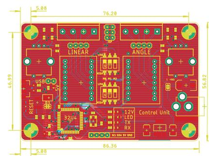
Figure 28. Dimensions of the PCB
