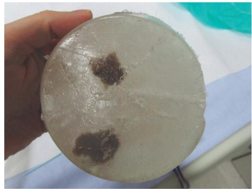
Figure 34. Phantom with traces of the needle
