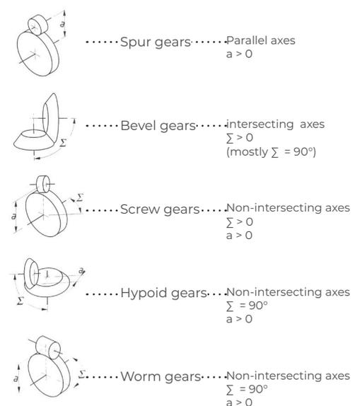
Figure 19. Different kinds of gears (Muhs et al, 2005)
