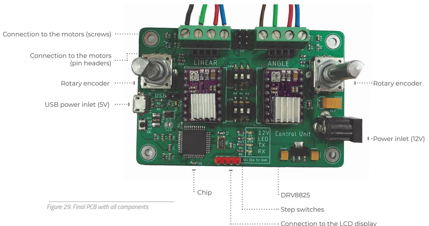
Figure 29. Final PCB with all components
