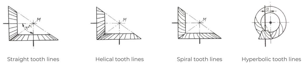
Figure 20. Hypoid gears with perpendicular axes (Muhs et al, 2005)
