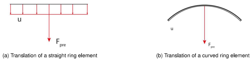
Figure 4.9: translation differences due to curvature in the ring elements prone to pre-tension
