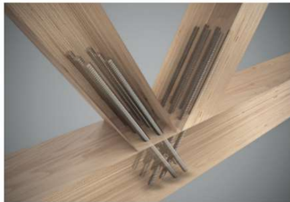
Figure 4.51: Glued in rods connection in a truss for the internal joints of the inner ring
