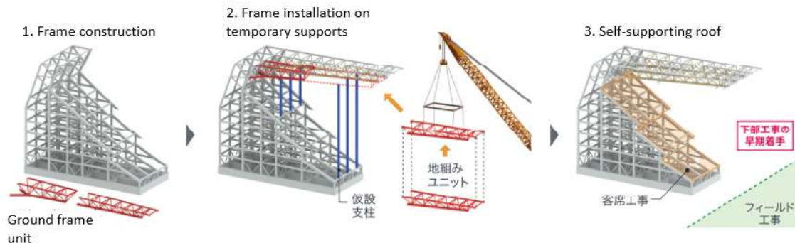
Figure 2.21: Construction sequence of the roof trusses
