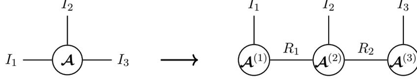
**Figure 3-3:** Diagrammatic notation of TT decomposition of a 3-way tensor  $\mathcal{A} \in \mathbb{R}^{I_1 \times I_2 \times I_3}$ .
