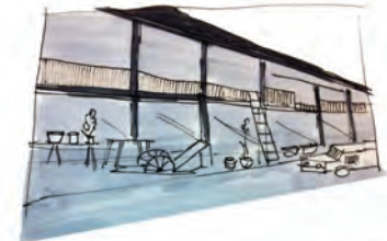
Fig. 9.39 The pole dwelling is a principle used worldwide. The shown building typology at the dwawing is found at the south east of Bangkok. The typology is well functioning in dry- and wet season and is constructed in groups of dwellings or as single dwellings.
