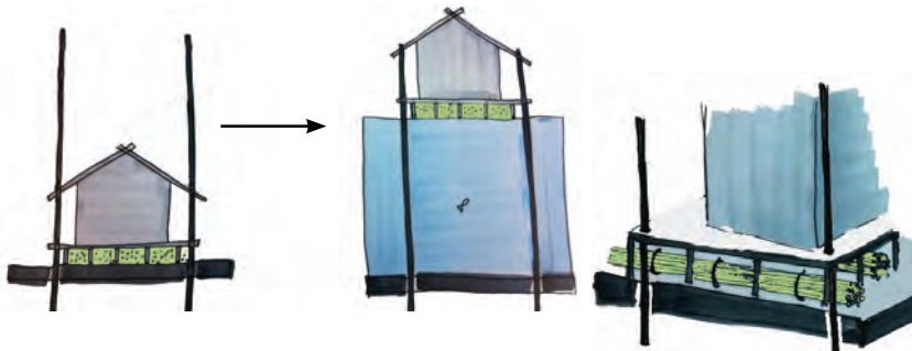
Fig. 9.38 This dwelling typology is found in Tha Khanon in Thailand. With the monsoons, the Khiriarat river overflows several times during the season what causes a flooding of 10 - 20 m height what can last for a few days till weeks. The whole community, including community center, is set afloat. The houses are placed on a bamboo construction and are constructed to stilts on the corners of each house (Jumsai, 2009).
