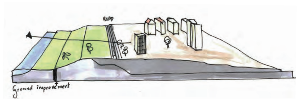
Fig. 5.7 Super levee Tokyo: Dike does not separate city - river and an urban park is integrated with the dike.
