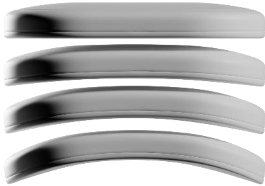
Figure 49 Sideview of bending prototypes in 0, 10, 20 and 30 degrees (top to bottom)
