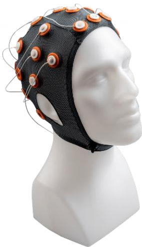
Figure 31 EEG using dry electrodes (Systems, 2025)
