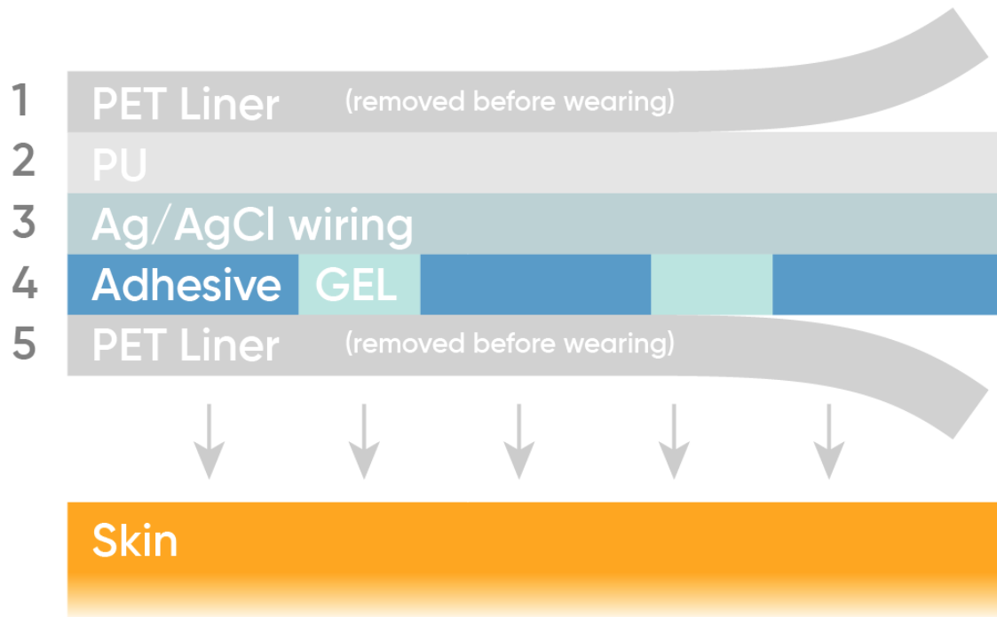
Figure 64 Basic ECG patch layering
