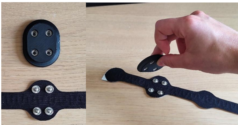
Figure 57 Enclosure directly connected to the patch
