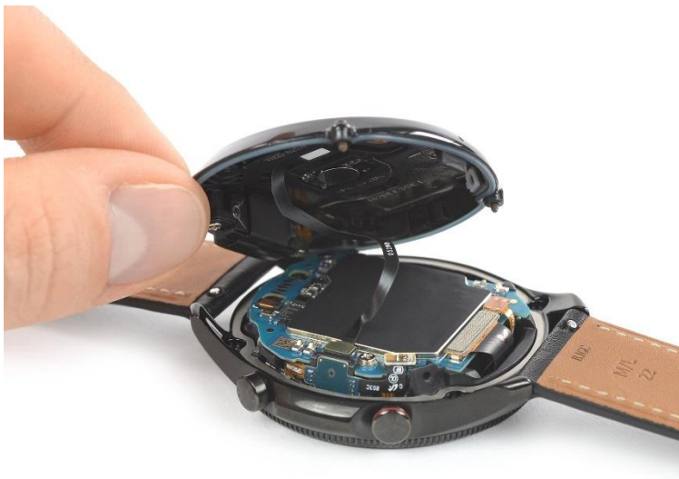
Figure 59 Galaxy Watch 3 opened up showing screws and a rubber gasket (Zwink, 2021)
