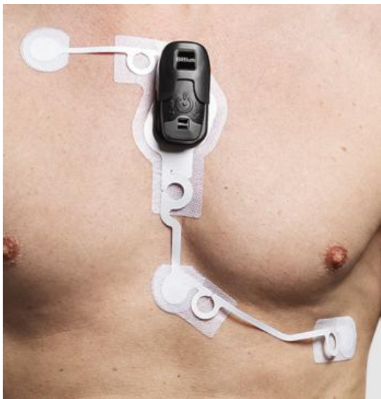
Figure 71 Straight conductive wiring on Bittium patch
