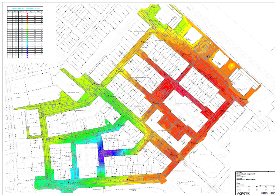
Figure G.17: Thickness of sand cover layer in Vogelweide, Diemen. Darkblue/ purple refers to a thickness of approximately 6-7 meters, green to approximately 3-4 meters, and red to approximately 1-2 meters. The image is acquired from an appendix of Te Groen (2016).
