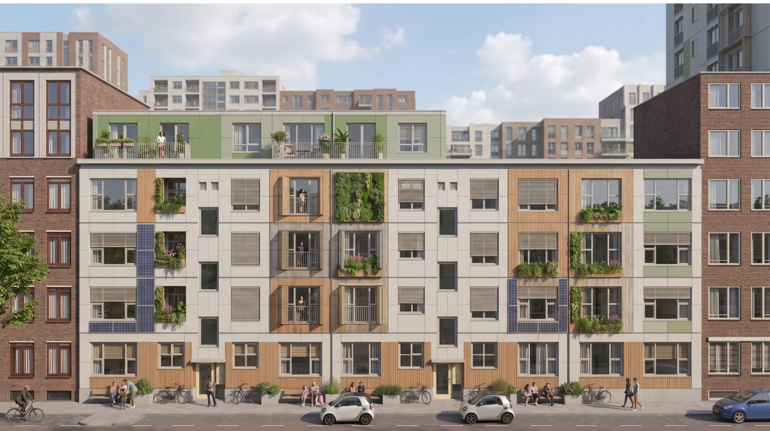
Figure 10.1 Speculative future scenario testing the framework against change (§10.6.6). The Layer 1 baseline and module grid remain fixed, while the resident-facing Layer 2 adapts to a changed social and technical world: added balconies, more greenery responding to resident needs, additional shading and BIPV to a warmer climate, and value-aware component substitution to rising material costs and supply constraints. An added rooftop storey, built in the same modular system, and taller neighbouring blocks reflect densification under housing shortage. The illustration shows adaptability achieved through Layer 2 reconfiguration rather than replacement of the whole envelope. (Conceptual illustration.)
