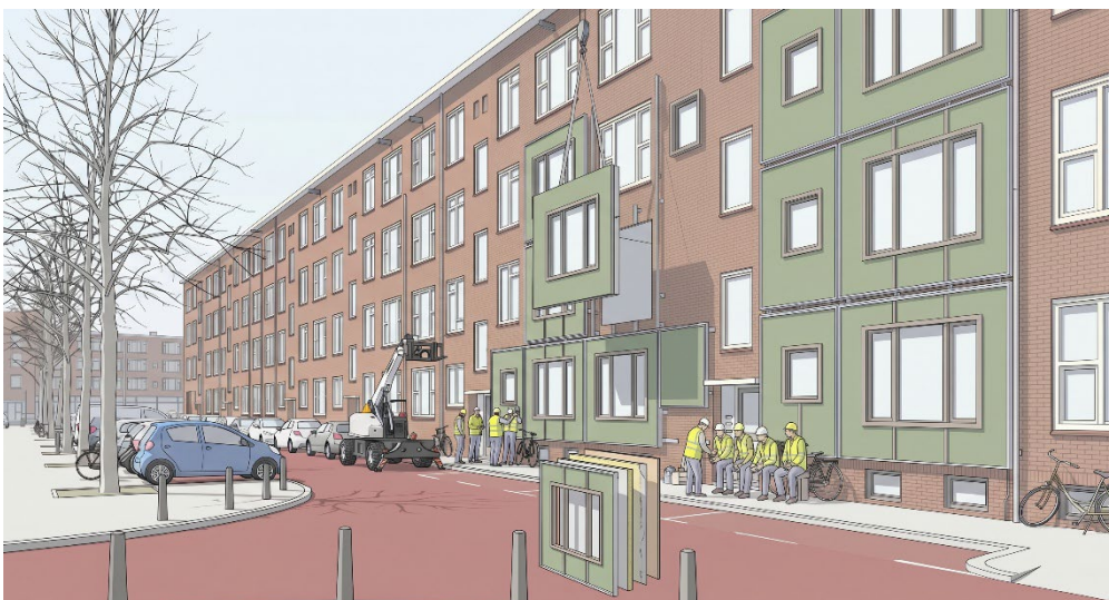
Figure 5.9: Schematic visualisation of base layer 1, applied on existing wall on site (own work)
