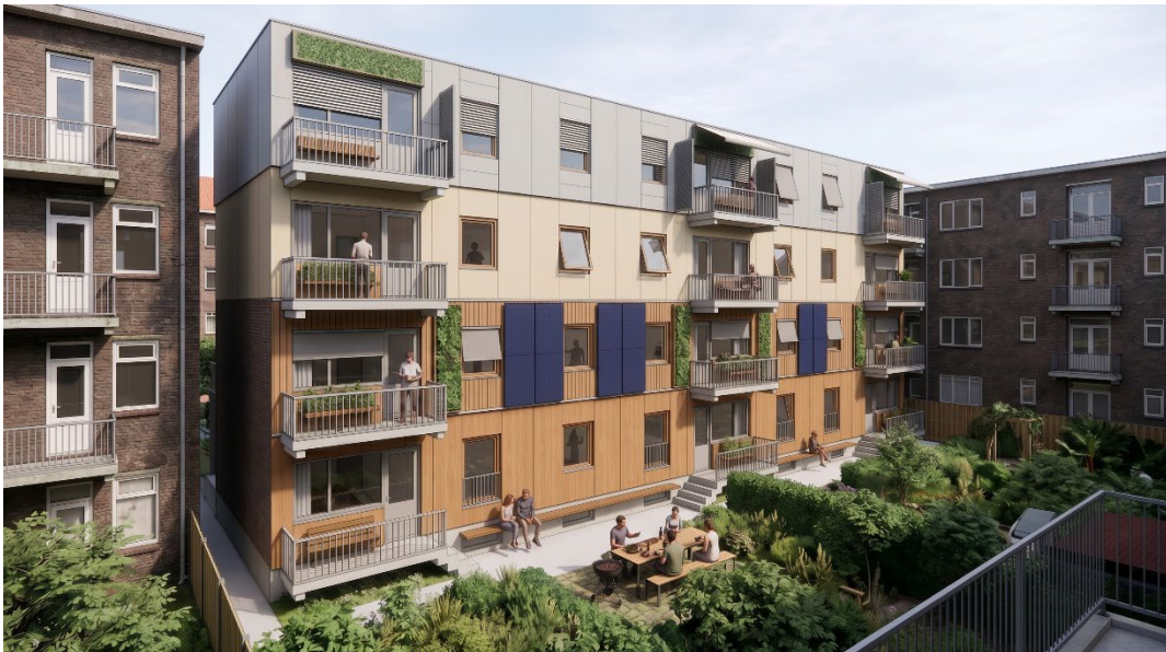
Figure 7.8: Facade design response design variant 01- north-street façade (only rockpanel and cariant 2 cladding south and noth combined, picture below south-courtyard facade including different variants (own work*)
