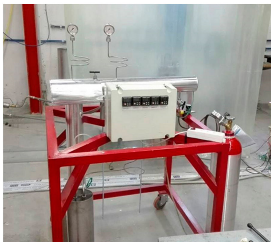
Figure 4. Experimental apparatus for CO 2 methanation process.
