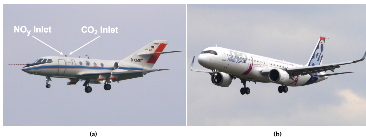
Figure 3.1: (a) Measurement platform Dassault Falcon 20-E5 (Registration: D-CMET) and (b) source aircraft Airbus A321-251NX (Registration: D-AVZO), equipped with two CFM LEAP-1A engines - adapted from internal source.
