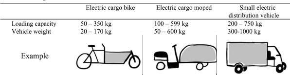
*Electric cargo bike*: an agile and active form of transport with a payload of up to 350 kilograms. Suitable for mail and parcel delivery services, food delivery and for services in which small volumes are delivered. However, designing for maximum payload could lead to compromises in the friendly character and maneuverability of the electric cargo bike.
