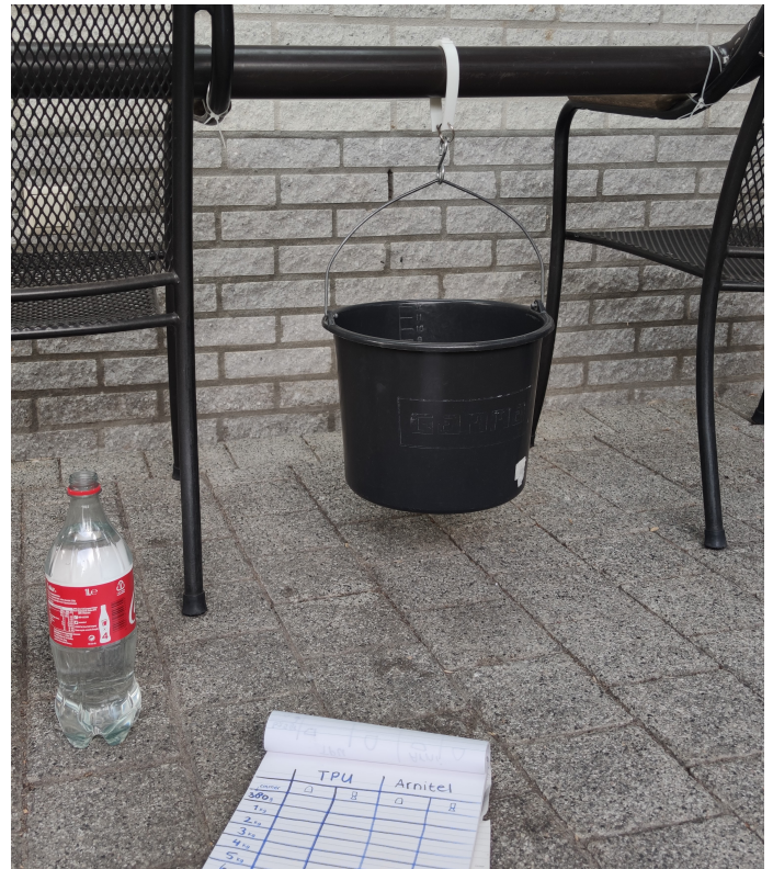
Fig. 20: Strength test 1: testing the materials and the performance of the spacer.
