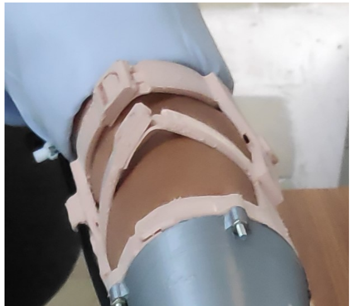
Fig. 5: Weak part of lock B, with a buckle in it.
