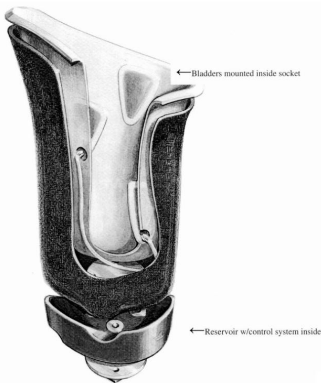
Fig. 18: Example of socket with liquid filled bladder: the Smart Variable Geometry Socket [42]
