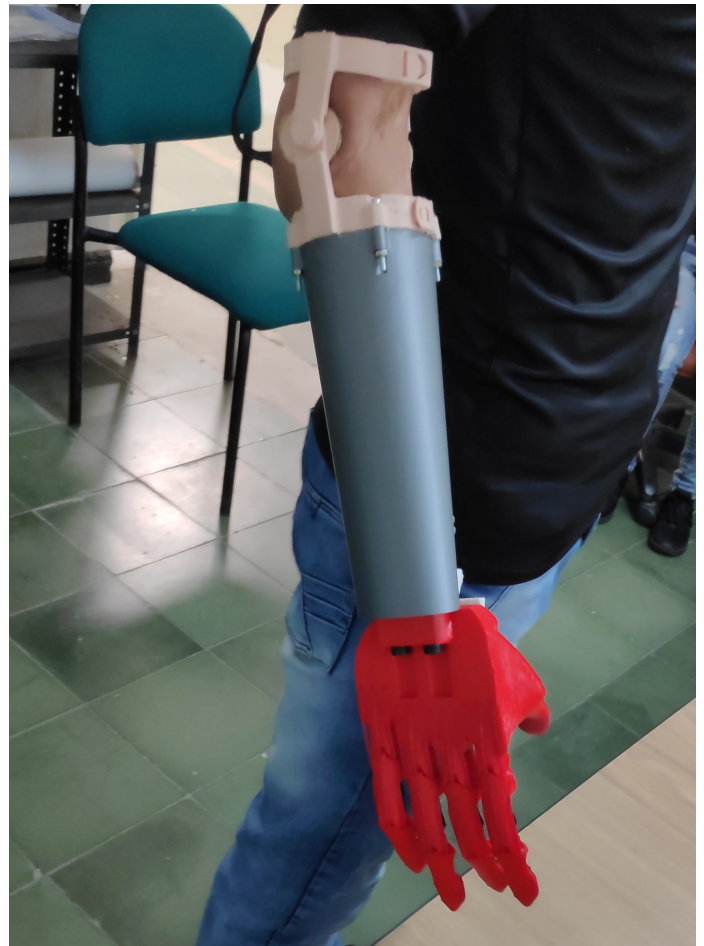
Fig. 4: The current 3D printed WILMER open fitting: a socket with hinges to connect the straps and to improve the range of motion.
