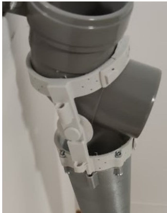
Fig. 23: Arnitel ID2045: the lower part of the socket was disconnected from the PVC pipe coil when a weight of 6 kg was applied to the end of the prosthesis.
