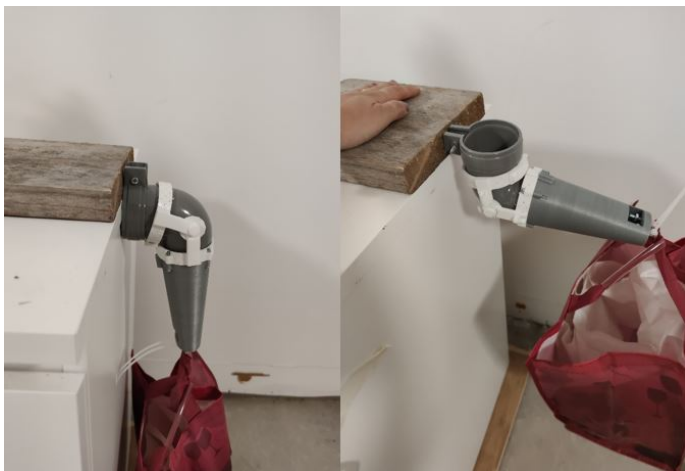
Fig. 22: Strength test 2: testing the performance of the complete socket. Set-up 1 (holding a bag with a shoulder abduction of 0^\circ ) and set-up 2 (holding a bag with an elbow flexion of 90^\circ ), respectively.
