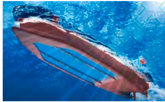
Fig. 14. A schematic diagram on the principle of the drag reduction through air layer [111].
