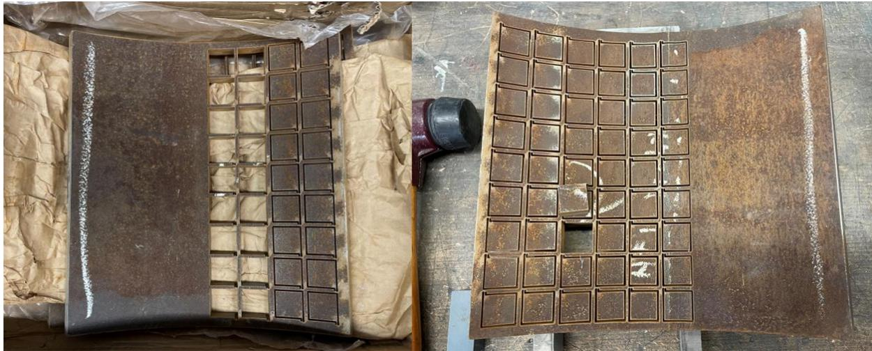
**Figure 36: H2ready X56 steel provided by Mannesmann Line Pipe GmbH. Interior sides with water jet cuts.**
