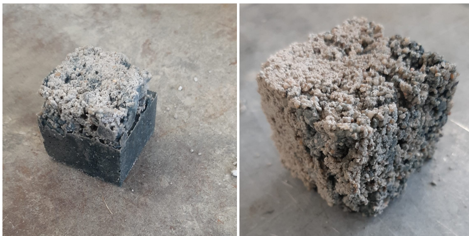
Figure 6.3: Poorly compacted mortar cubes from mix D (left) and E (right).
