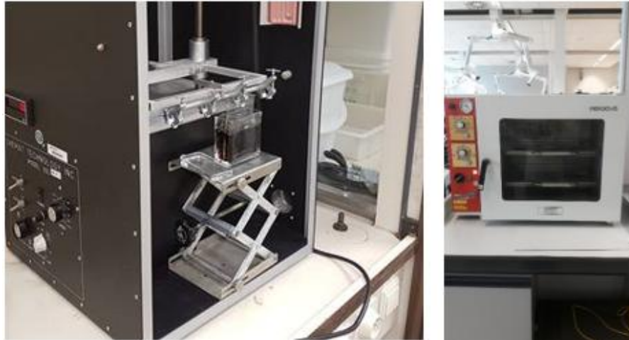
Figure 4.8. DipMaster 201 and Heraeus D-6450 Hanau oven (Photo credits to Dr. Aike Wypkema and Natalya Tsoy)
