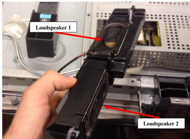
**Fig. 6.** Closer look of the TV loudspeaker assembly, and the location of the two loudspeakers.
