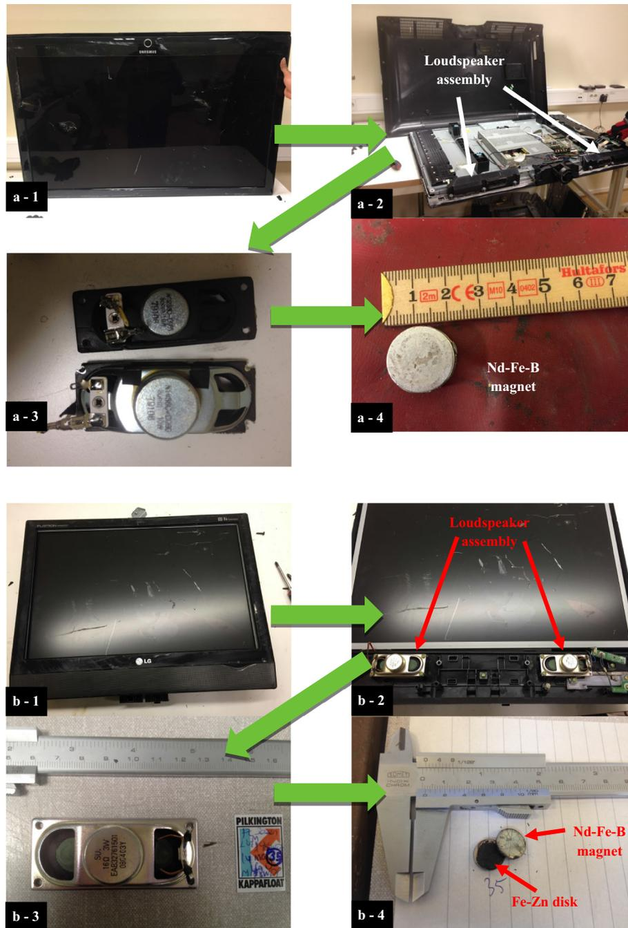
Fig. 5. Exemplification of the disassembling process and the location of the loudspeakers/Nd-Fe-B magnets for flat TV (a: 1–4) and PC screen (b: 1–4).
