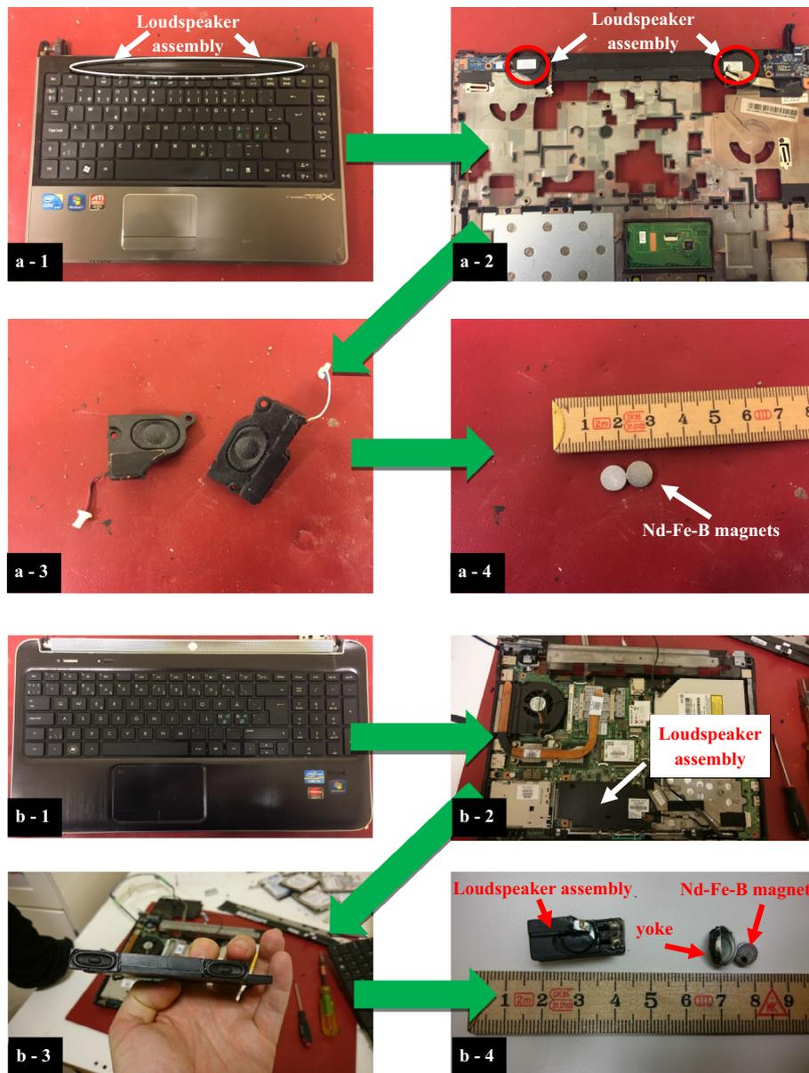
Fig. 3. Example locations of loudspeakers in laptops: (a: 1–4) beneath the laptop screens or (b: 1–4) under the keyboard.
