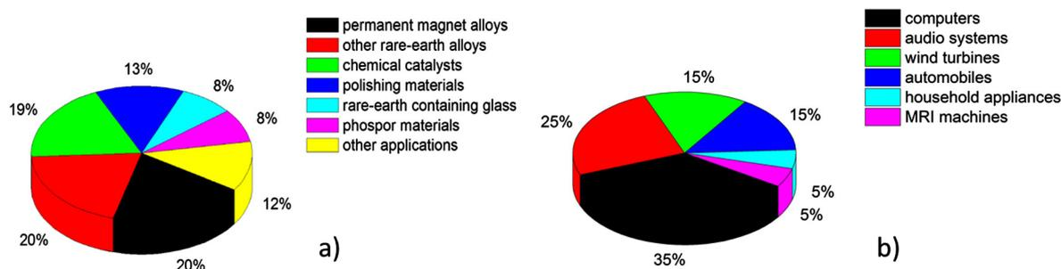
Fig. 1. Industrial use of mined REEs (a) and applications of Nd-Fe-B permanent magnets (b) (Wübbecke, 2013; Du and Graedel, 2011).
