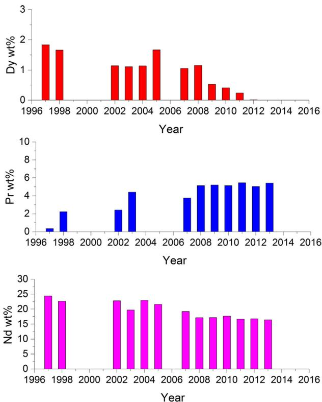
**Fig. 4.** Content evolution of the Dy, Pr and Nd in loudspeaker magnets collected from laptops.
