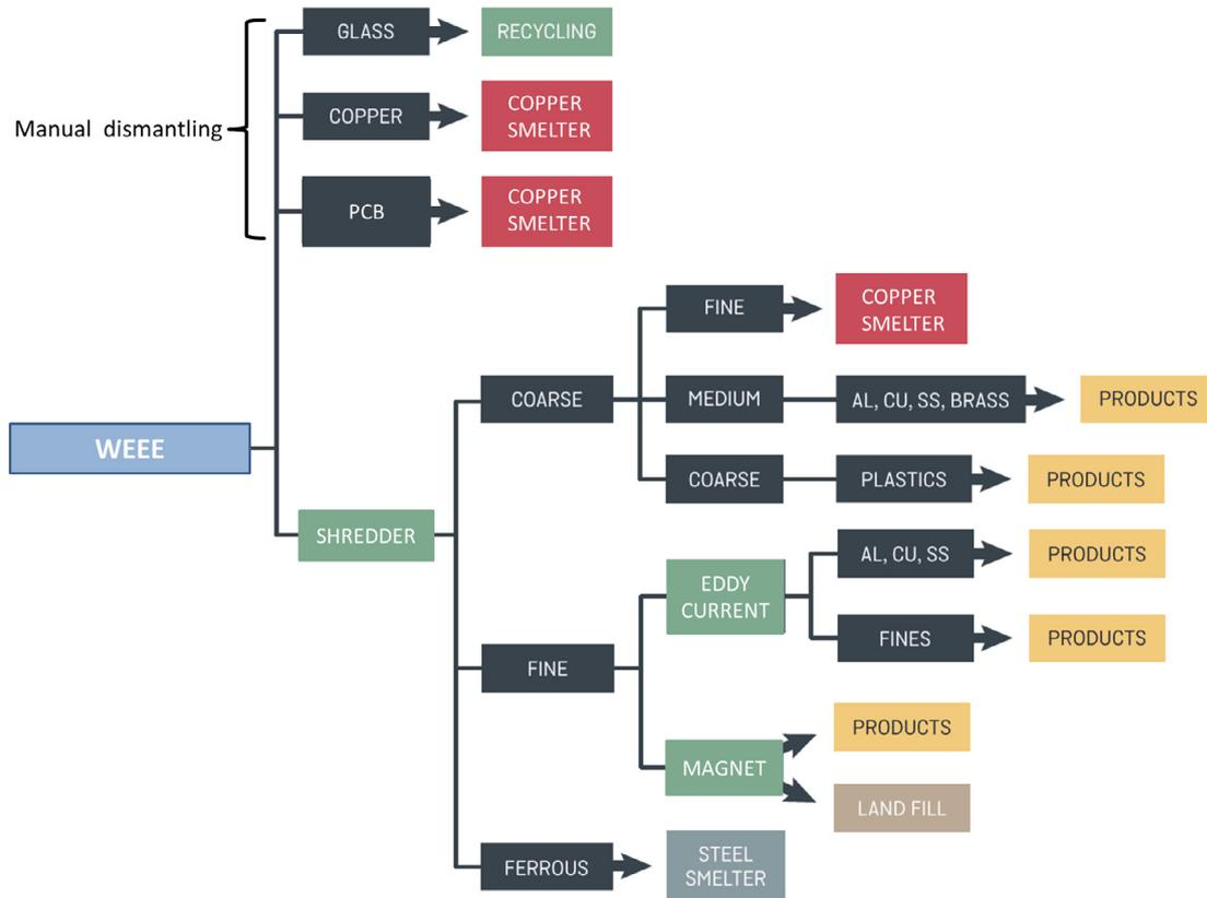
Fig. 2. Diagram of the sorting and recycling process developed at Stena Technoworld's WEEE recycling plant.
