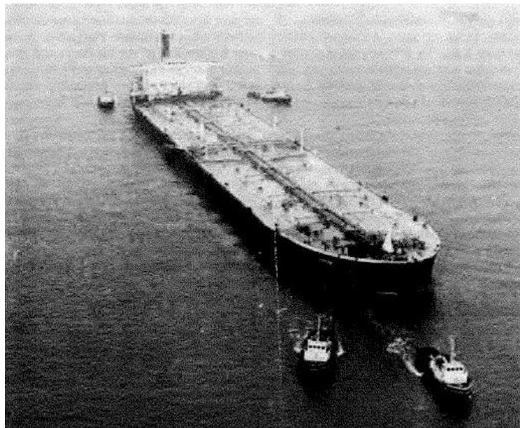
Figure 2: The 318t deadweight oil tanker SS Lepton was a subject of investigation for the full scale experiment at the Port of Rotterdam in 1974. Here, SS Lepton is filled with water enters the Port of Rotterdam. Observers on board carefully follow the sailing behavior of the ship.
