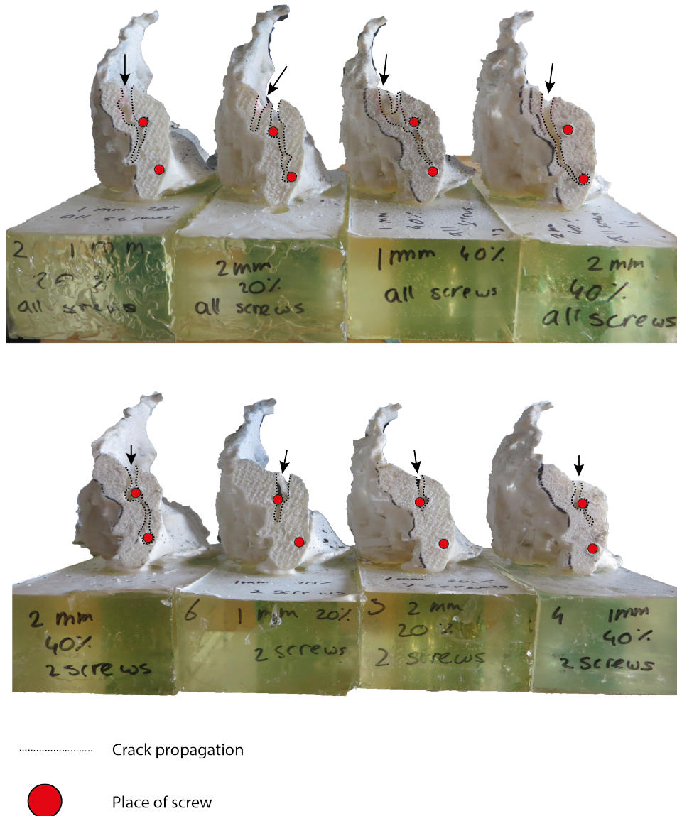
Figure 3.6: Crack propagation for all screws inserted (top) and 2 screws inserted (bottom). Dashed black line indicates crack and red circle indicates place of screw insertion. Initiation of crack in the models with all screws inserted is behind the lower side screw, while for the models with two screws inserted the crack initiates precisely at the height of the lower side screw (screw 5).
