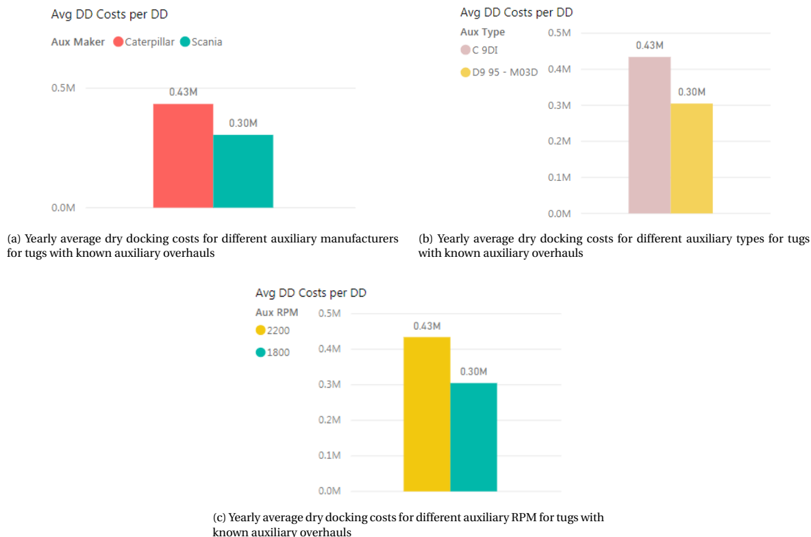
Figure 10.37: Detailed evaluation of auxiliary engine manufacturers, auxiliary engine types and RPM
