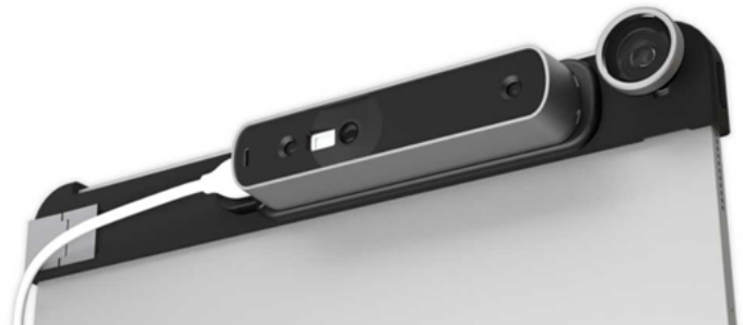
Fig. 5a: The Occipital Structure Sensor Mark 1 shown with the attachment bracket and the iPad.
