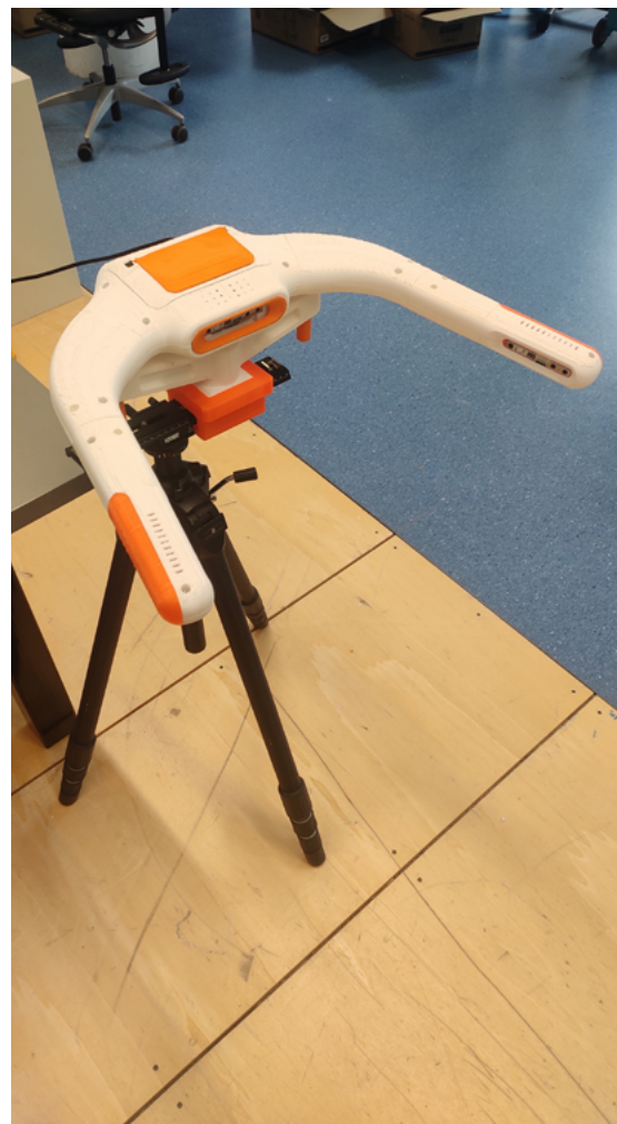
Fig. 14c: A working prototype of the Head-scanner complete with the mount and color scheme.
