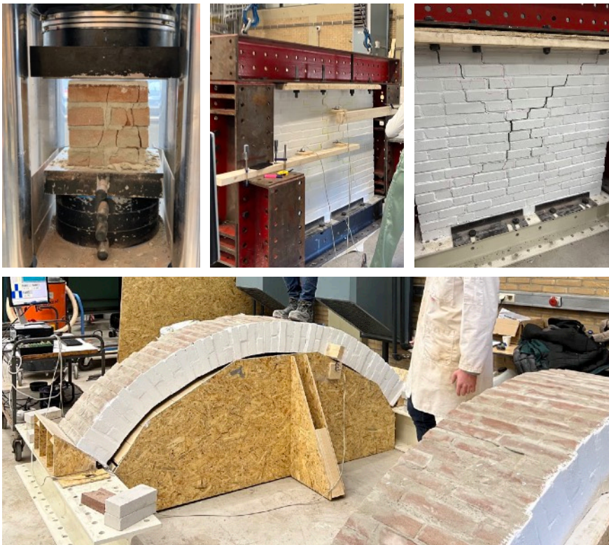
Figure A.10. Various experiments from the course, featuring a compressive test on masonry, a wall tested out-of-plane, with vertical and horizontal cracking, and an arch.
