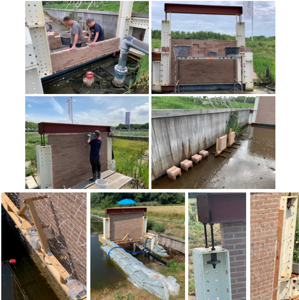
Figure A.7. Collage detailing the construction and context of the tested wall.
