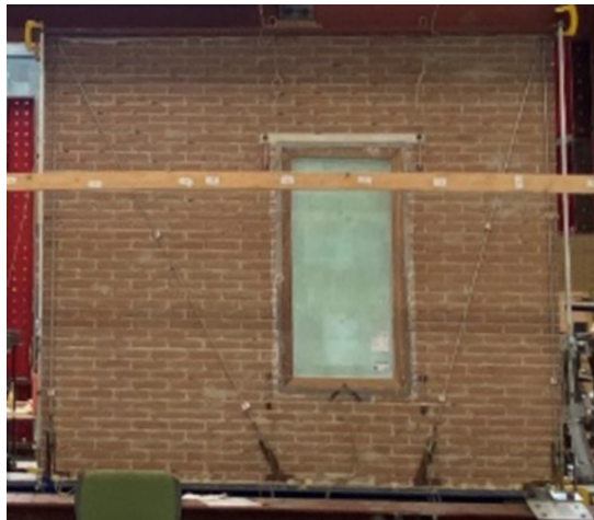
Figure A.5.1. Experimental masonry wall with window of timber-glass design. The glass is painted for DIC purposes.
