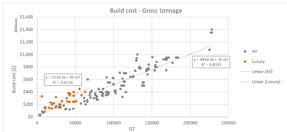
Figure 7.8: New build cost as function of GT for luxury cruise ships and all cruise ships
