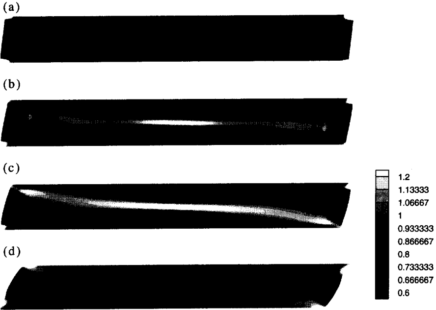
Fig. 5.16. Contours of normalized plastic shear strain \gamma^p/\Gamma^p for the specimen with B_0/A_0 = 7.5 at various deformation stages: (a) \Gamma = 0.12 , (b) \Gamma = 0.20 , (c) \Gamma = 0.30 , (d) \Gamma = 0.71 . The material parameters are as in Fig. 5.2.
