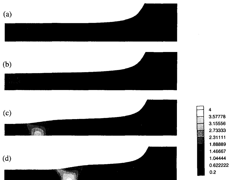
Fig. 6.11. Contours of normalized plastic strain rate \dot{\Sigma}^P in the case of no intrinsic softening but with an apparent softening under plane strain tension at various deformation stages: (a) \epsilon = 0.09 , (b) \epsilon = 0.16 , (c) \epsilon = 0.30 , (d) \epsilon = 0.43 . All figures are scaled to the same apparent specimen length.
