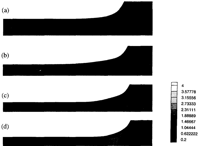
Fig. 6.7. Contours of normalized plastic strain rate \dot{\Sigma}^P in the case of no intrinsic softening nor permanent softening under plane strain tension at various deformation stages: (a) \epsilon = 0.09 , (b) \epsilon = 0.38 , (c) \epsilon = 0.53 , (d) \epsilon = 0.60 . All figures are scaled to the same apparent specimen length.
