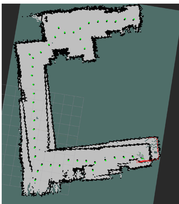
FIGURE 10 Drift in the map where the hall is doubled. The drift occurred 10 min after the autonomous navigation started in trial 3.
