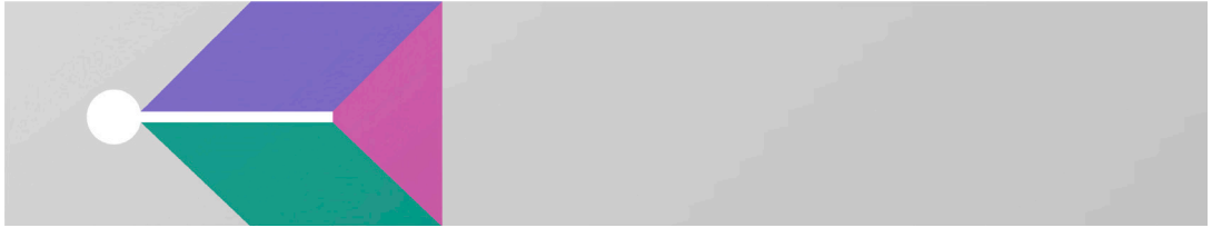
Fig. 11. Patch decomposition of the fluid domain for the FSI2 benchmark. The rigid cylinder (white disc) and the elastic beam (white strip) form the inner obstacle. Three colored patches conforming to the cylinder-beam interface (purple, magenta, and green) constitute the regenerated region: at every coupling iteration these patches are reparameterized to follow the deformed beam, using the barrier-patch construction of Section 3.2. The remaining gray region is covered by frozen extension patches that span the rest of the channel up to the inflow, outflow, and wall boundaries; these are generated once and remain fixed throughout the simulation. Confining the regeneration to a narrow neighborhood of the beam keeps the per-iteration meshing cost essentially independent of the channel length. (For interpretation of the references to color in this figure legend, the reader is referred to the web version of this article.)
