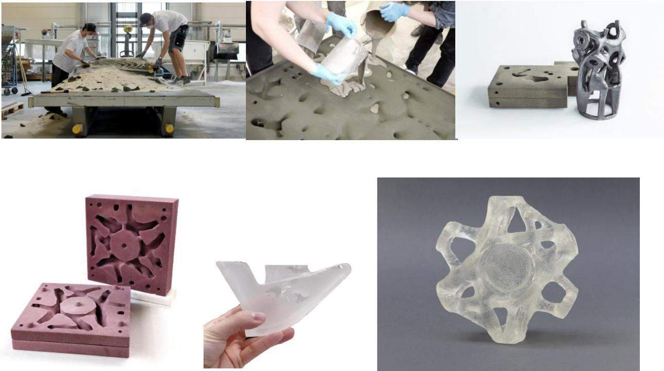
Figure 16 3d-printed sand moulds used for the casting of (top left & middle) concrete slab, (top right) steel node, (bottom left & middle) cast glass node and (bottom right) cast glass prototype.
