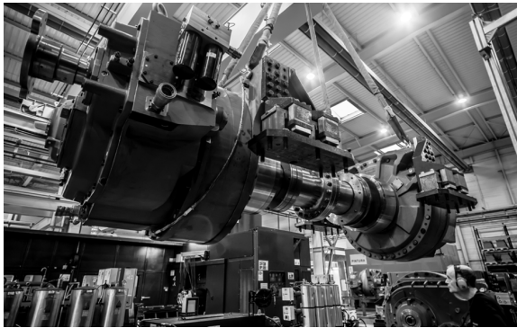
Figure 2. Lift operation of two gearboxes.
