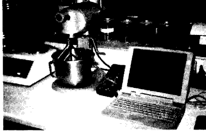
Picture 6.1 Mixer and electric power measuring device
