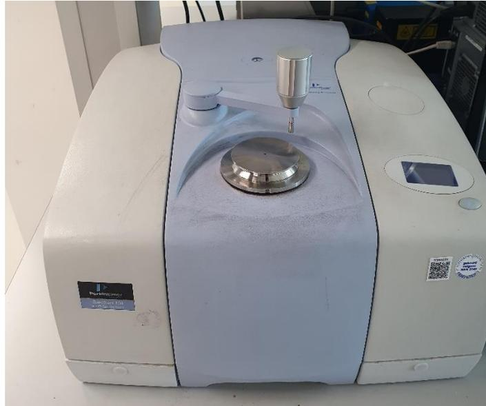
Figure 27: Spectrum 100 FT-IR spectrometer
