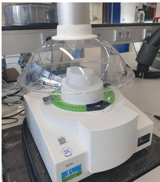
Figure 25: TGA4000 thermogravimetric analyser
