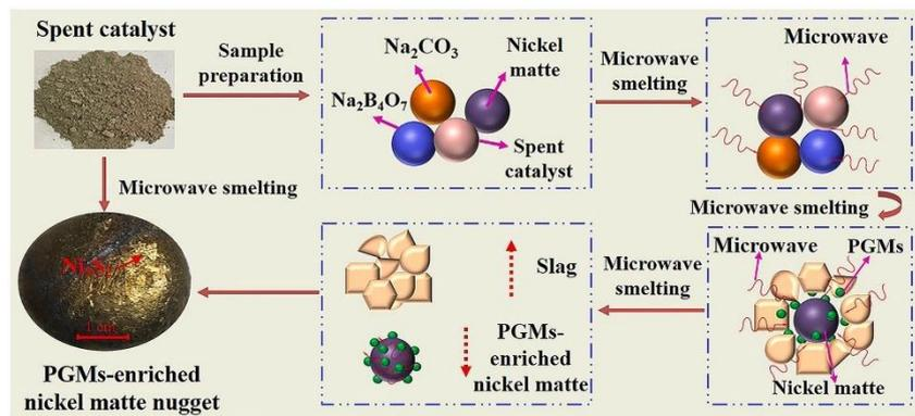
Figure 45: Microwave assisted smelting (Source: [124])
