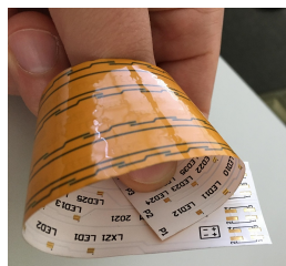
Figure 4.6: Flexibility of the LED-sheet.
