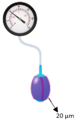
Figure 1.28: Experimental setup of a concentric, 20\mu\text{m} thick LCE wrap surrounding a balloon with air. Stimulation of the LCE wrap results in a concentric contraction, increasing the pressure inside the balloon, which is displayed on the pressure gauge. This experiment was done to simulate LCE influence on ventricular pressure when used as cardiac assist device. The LCE wrap was able to generate a high normalized pressure compared human cardiomyocytes for the same layer thickness (pressure shown for 1mm thickness). A light stimulus of 50\text{mW}/\text{mm}^2 with activation pattern ( t_{on}/t_{off} ) of 200/800 ms was used (60bpm) [55].
