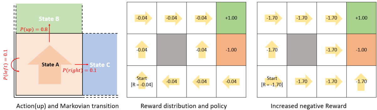
Figure 4.9: MDP explanation, left: Markov transition principle for MDP and right: two reward distributions with corresponding policies
