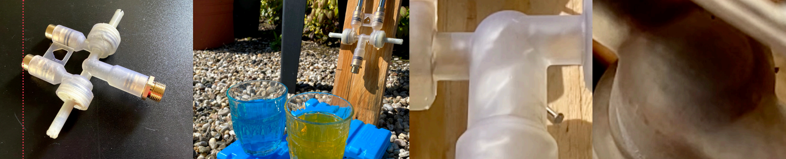
image [35] Testing setup and images showing the swirling motion inside of the mixing chambers
