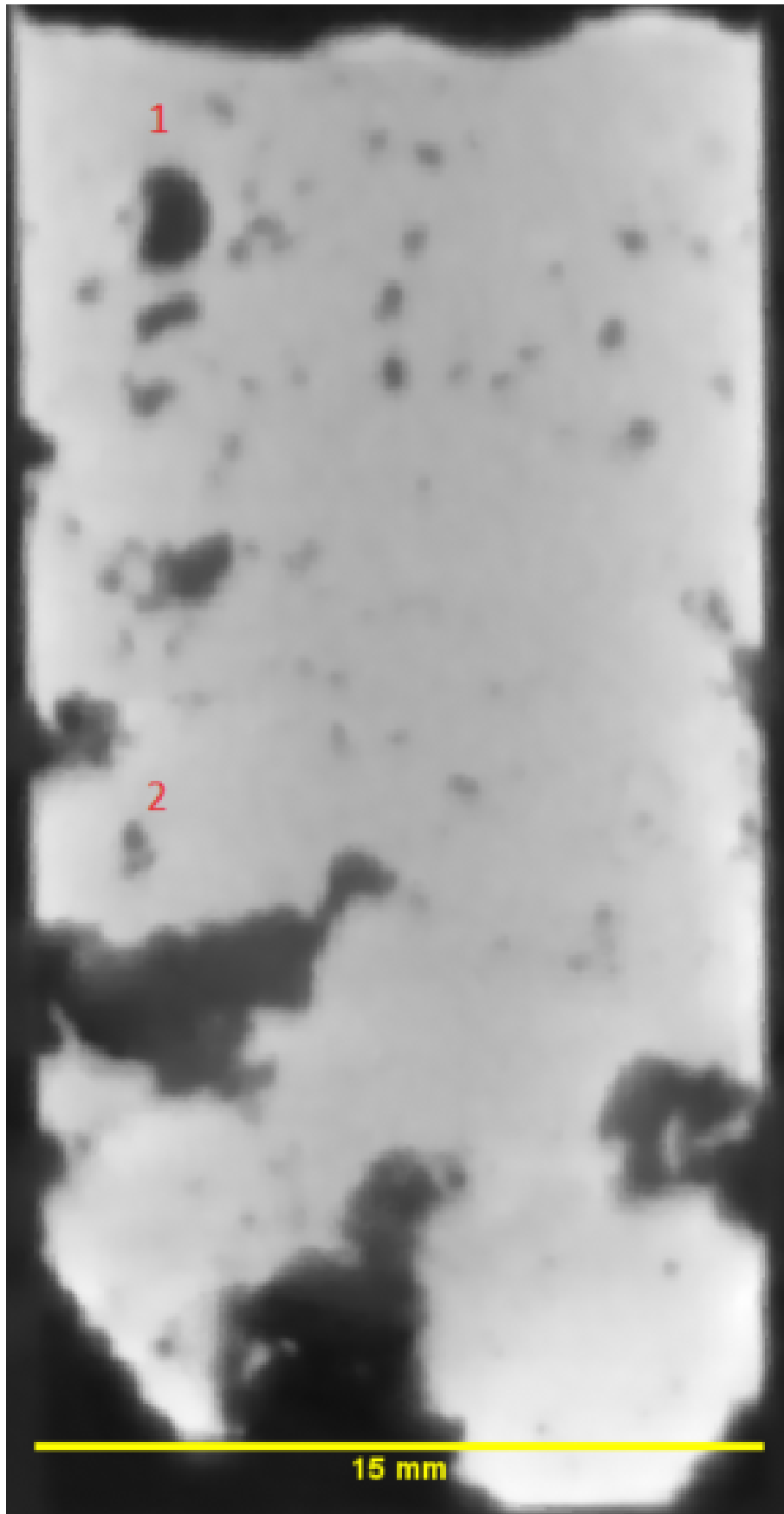
Figure 34: Labelled pore on tomographic image which represents a fibre filled with air; The greyish bulk is the peat material between the fibres which is a mixture of heavy water, natural water and decomposed plant tissue
