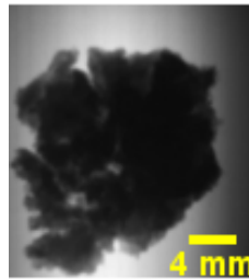
Figure 27: Neutron radiograph of Uitdam peat with its natural water content stored inside a container made of aluminum foil Diameter : 1.5 cm and Wall thickness: 0.12 cm
