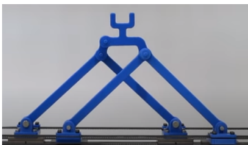
(g) 2D linear parallel manipulator with kinematic redundancy by Gosselin et al. [13]
