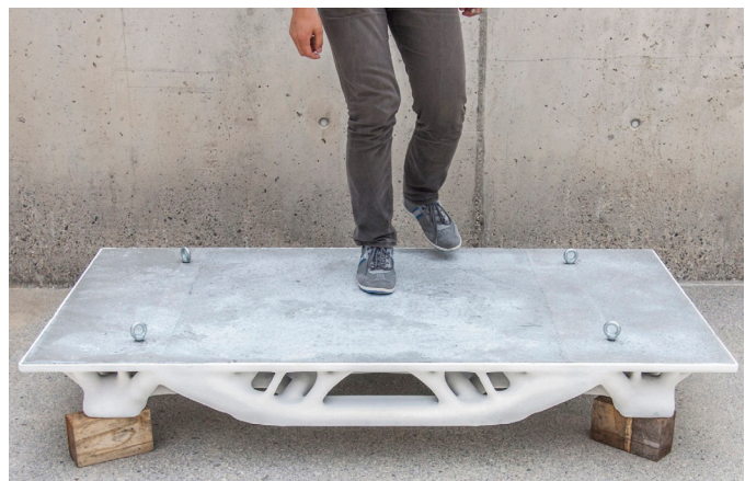
Image 13: Left: Element being constructed using the Stay-in-Place formwork technique. Right: Result 16
