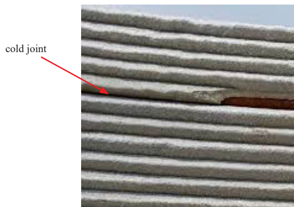
Image 15: Formation of a cold joint 20
