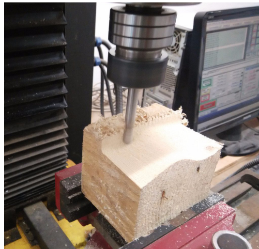
Image 7: Wood mould being carved with a CNC milling machine 10
