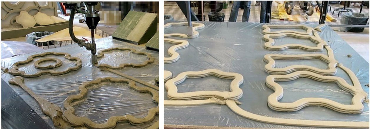
Image 11: Element being 3D printed using the Fleximould technique 14
