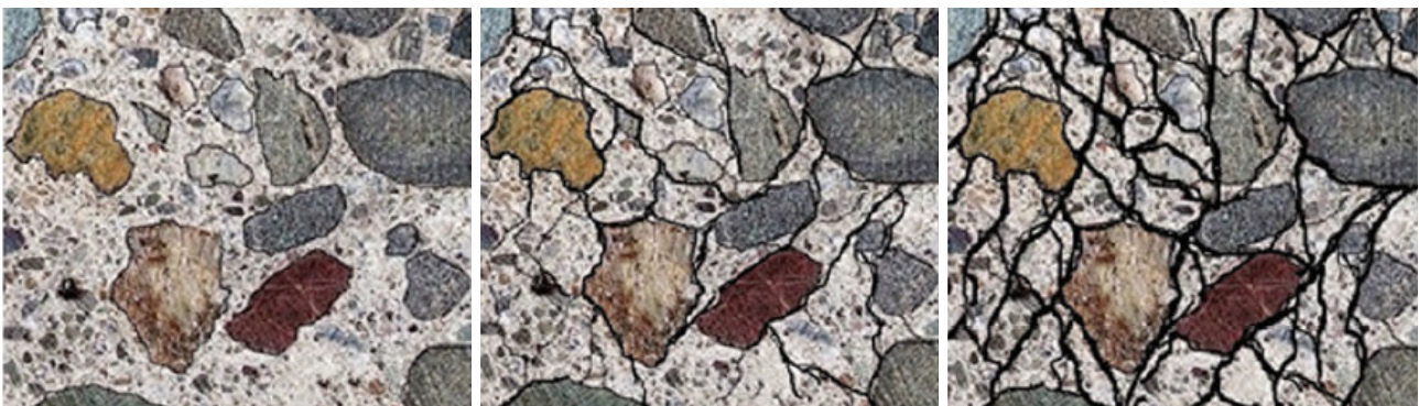
Image 5: Crack forming from interfacial transition zones 8
