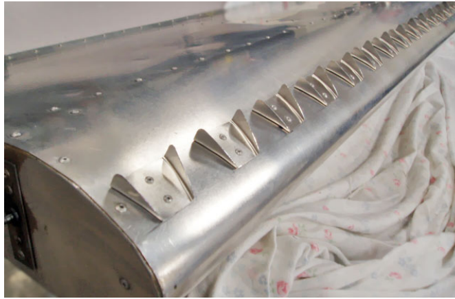
Figure 2.26: Example of vortex generators in pairs on wing [59]
