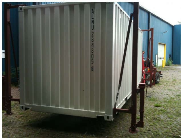
Figure 4.2: Manual container lifting device [86]
