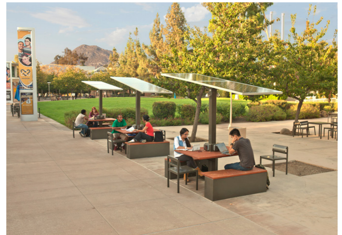
Figure 16: "Off-grid Solar-Powered Charging Stations" (Innes, 2017)
