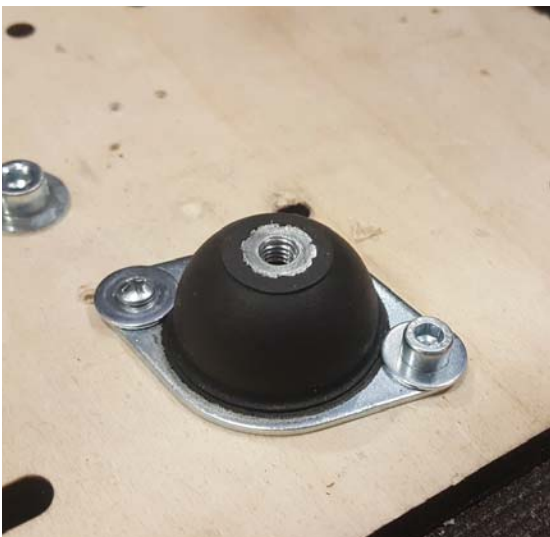
Figure 58: Several purchase rubber damping elements were used, such as dome mounts and ring mounts.
