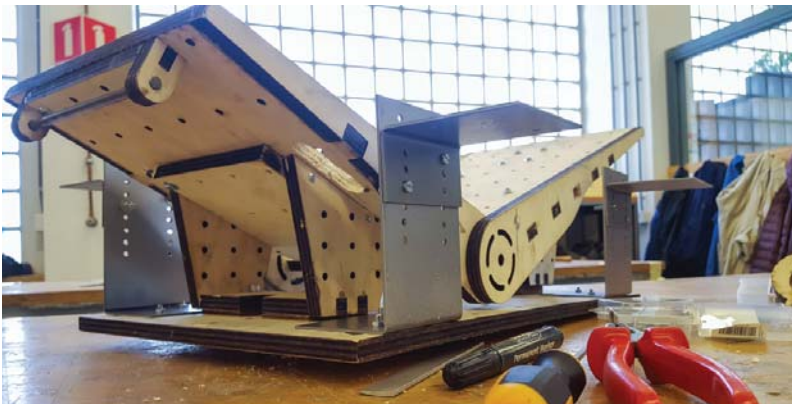
Figure 69: Canned aluminum brackets were attached to the 'interface surface'. Yet, they were considered to be not stiff enough and might have resulted in a certain degree of resonance.
