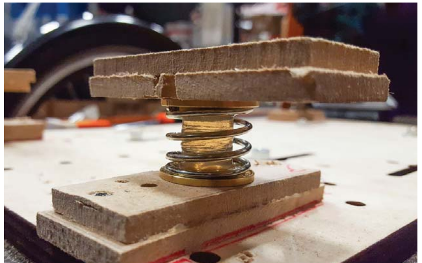
Figure 72: This type of isolator used a coil spring together with a solidified silicone gel for damping.
