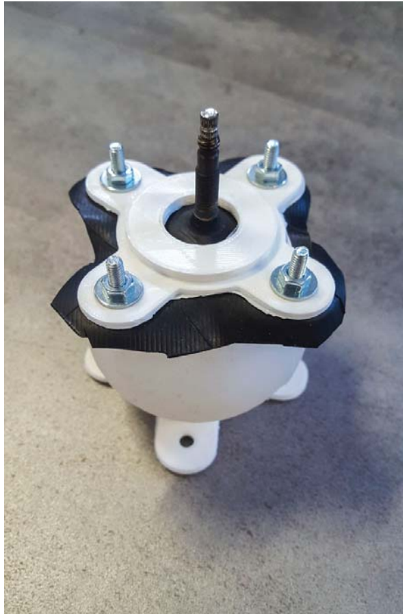
Figure 57: Possibilities were being evaluated to make rubber damping balls airtight. This would create some sort of air suspension.
