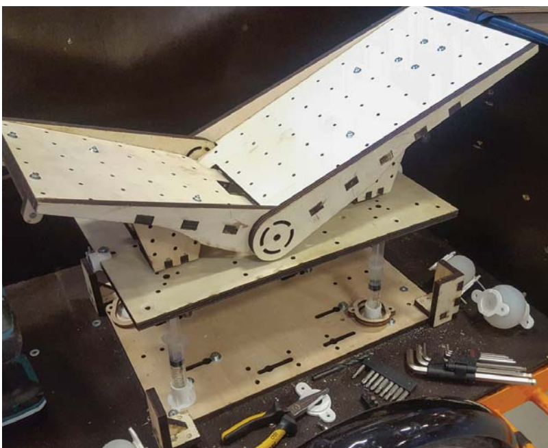
Figure 64: Syringes in different volumes were used. Syringes are rigid elements and cannot expand in volume (as opposed to a balloon, e.g.). The damping of these elements make use of air pressure change and no volume change as normal air suspension does.
