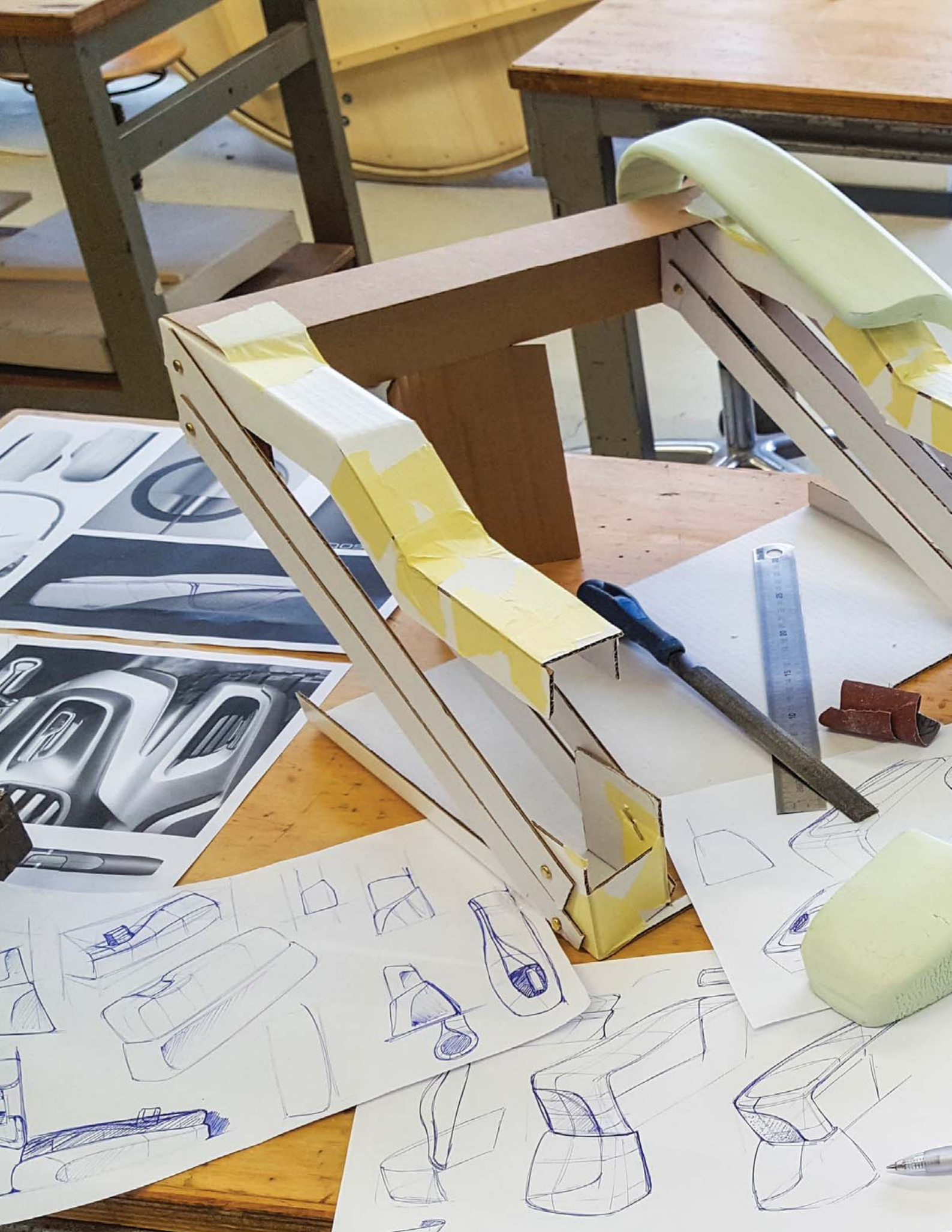
▲ Figure 120: Cardboard representation of the construction. Foam shapes were formed that could be placed on top of the construction. The same side profile (a smooth waving curvature) was used for all foam models. The sketches that formed the starting point for the foam models are displayed on the table as well.
