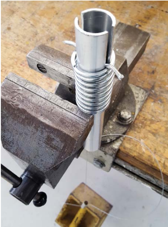
Figure 61: Test set-up to validate the spring rate, consisting of an incised aluminium tube and a bent nail that moved in the incision.
