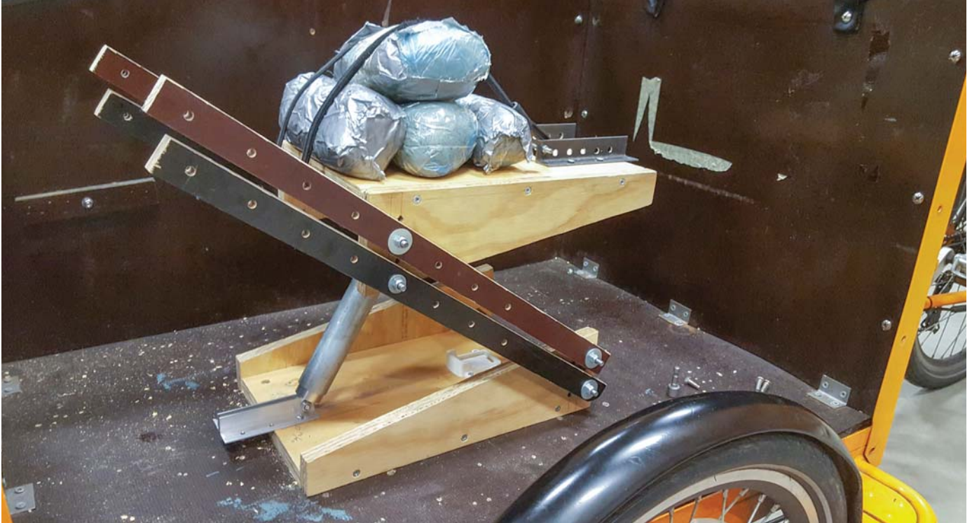
Figure 144: (bottom right) Wooden test model loaded with a 8-kg test dummy
