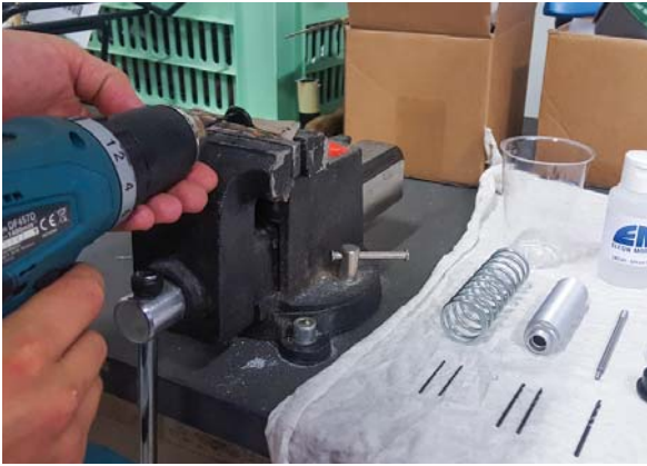
Figure 66: In order to let the shock absorber react precisely to bumps in the road, both holes of the piston were drilled larger in steps of 0.5 mm after each test.
