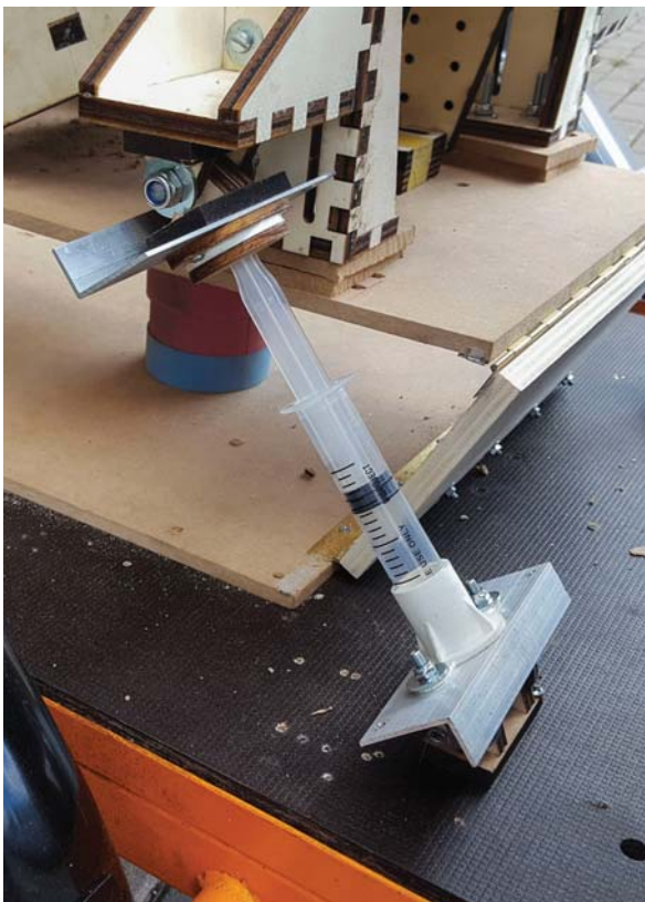
Figure 74: Placing the syringes next to the platform resulted in a lower center of gravity, thus creating more stability.
