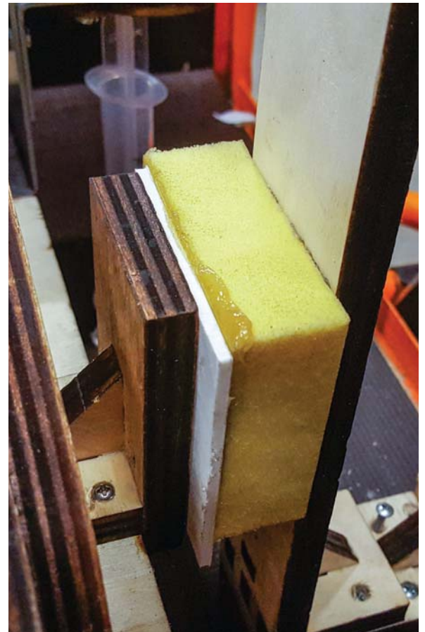
Figure 70: Friction damping between a plastic and foam surface. Lubrication was added to smoothen the friction.
