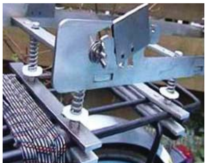
Figure 25: (middle) The Traveljack is mounted to the handlebars, making cornering heavier.
