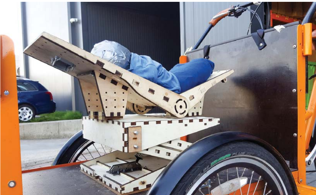
◀ Figure 47: (upper) Platform construction. Here, mounted with inclined rubber damping balls.
