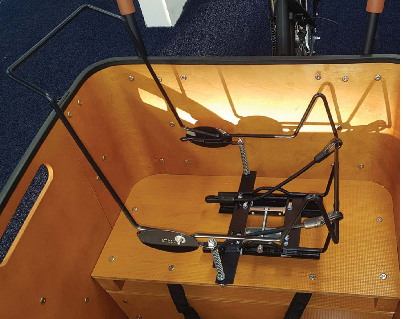
▲ Figure 21: The Steco Baby Mee adapter can be fastened to the majority of cargo bikes and can be placed on the bench or on the floor of the cargo bike. The infant safety seat is fastened to the Steco Baby Mee by means of two elastic bands.
