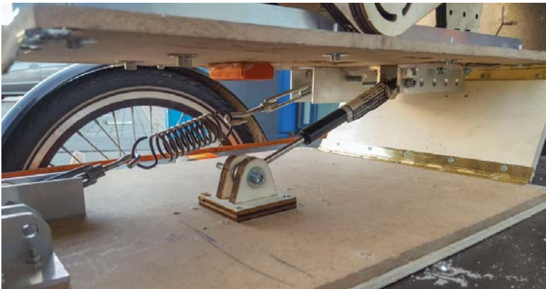
Figure 68: A gas spring pushes with a constant and preset force. Whether the system worked, depended on the resulting force between the gas spring, the tension spring and the weight that was laid on the parallelogram.
