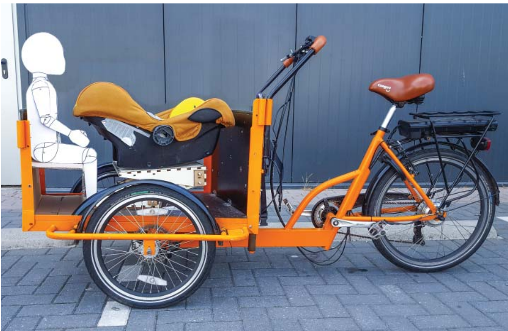
Figure 86: (upper) Mannequin showing the child's knees might become entrapped by the low positioned infant safety seat (8 kg's included)
