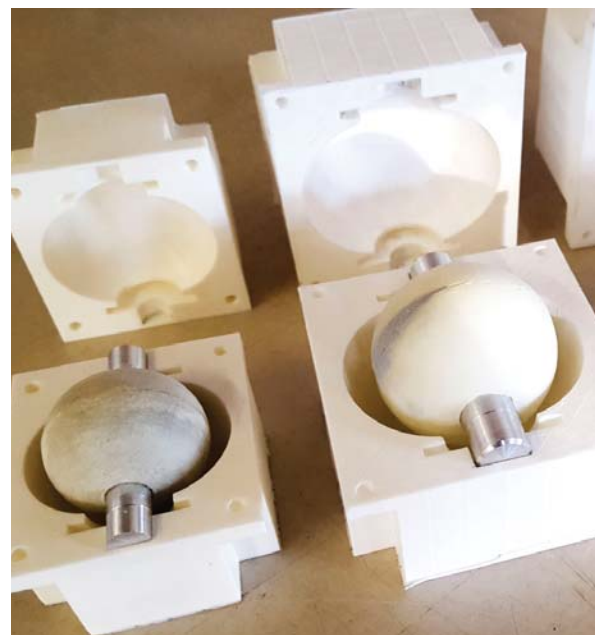
Figure 78: small, medium and large rubber damping balls were poured with self-made molds.
