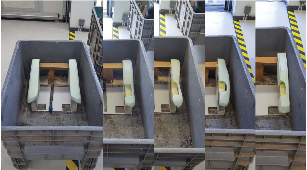
▲ Figure 121: The construction and foam shapes were placed in a grey box and photographed. In Adobe Photoshop the shapes were mirrored. By doing so, the look and feel of the product, when placed on the floor of a cargo bike, could be simulated rather well.
