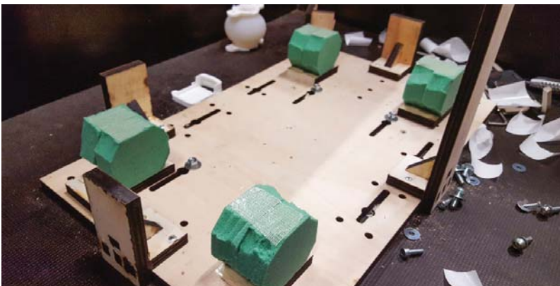
Figure 56: Out of a Regufoam® foam plate, multiple hexagons were cut that served as damping material. The vertical wood construction on the sides served as guidance.
