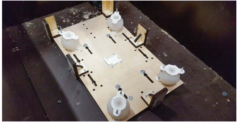
Figure 67: Four rubber damping balls were placed at the corners of the platform construction. Inspiration was found from drones that use rubber damping balls to stabilize camera images.
