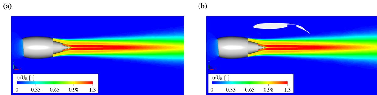
**Fig. 6 Time-averaged  $x$ -velocity contour plots for isolated and installed jets without free-stream**
