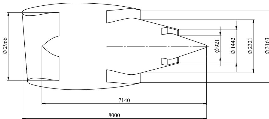
Fig. 1 GE90-94B engine cross-section and dimensions (in mm)
