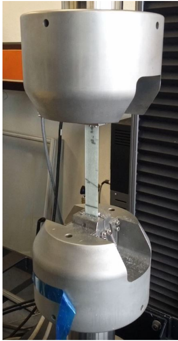
(a) Tensile testing in progress, note that the extensometer has already been removed.
