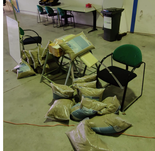
Figure 10.4: Failure of static test article
