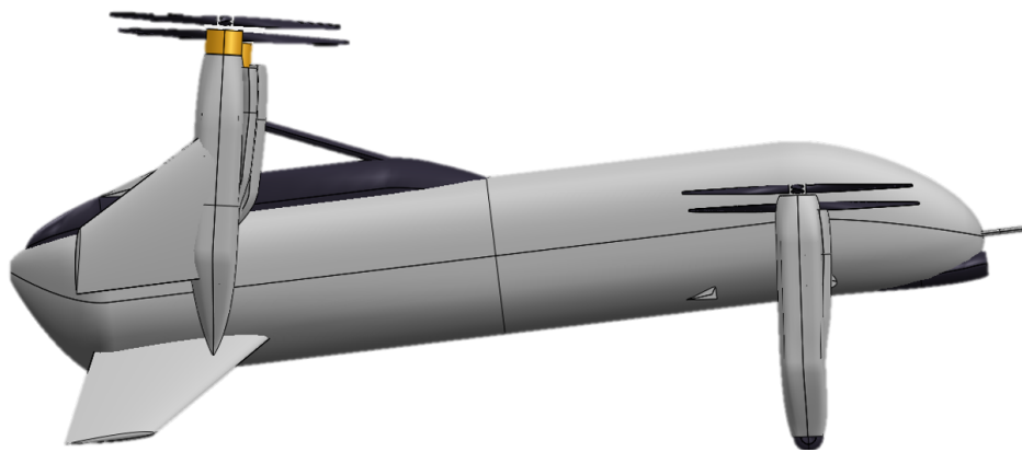
Figure 3.4: Concept 3: Sitting on the ground in hover configuration.
