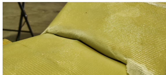
Figure 10.6: Detailed picture of the primary failure mode: local buckling which caused collapse of the structure.
