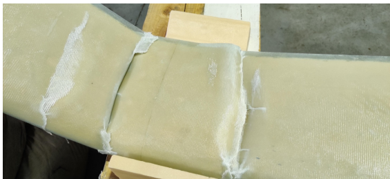
Figure 10.5: Damage on the static test article. Visible on the top side of the wing, flipped right side up. From left to right; Secondary failure - primary failure (buckling) - secondary failure.
