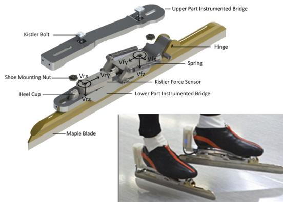
Figure 3.2 Overview of the instrumented bridge and an attached blade. The lower part of the bridge is only attached to the blade via the hinge. The upper part of the bridge is attached to the lower part via the Kistler bolts under pre-stress. The skater can place its own shoe on the bridge via the Shoe mounting nuts. The small white box near the heel is the recording and transmission unit for the measured data.
