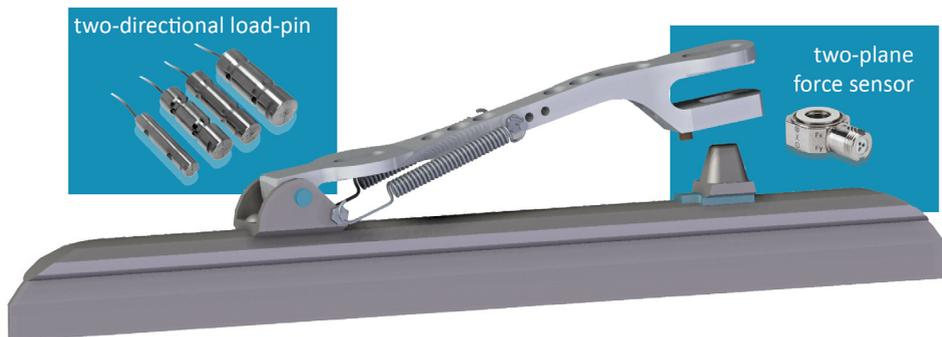
Figure 10.3 Possible design in the future: replacing the hinge by a two-directional load pin, and placing a load cell under the heelcup of the skate.
