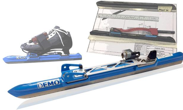
Figure 10.1 New design instrumented Klapskates.
