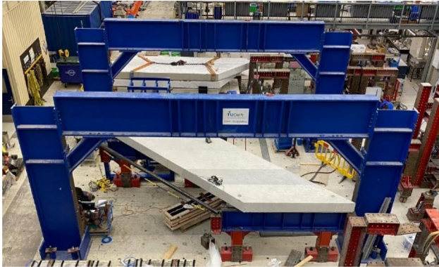
Figure 11. Skewed slab testing at Delft University of Technology.
