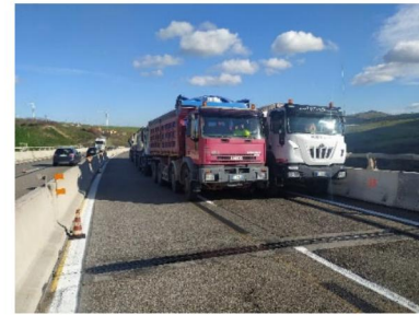
Figure 10. (a) Plan view of the proof load layout for the case study bridge; (b) picture of the eight loaded dump trucks.
