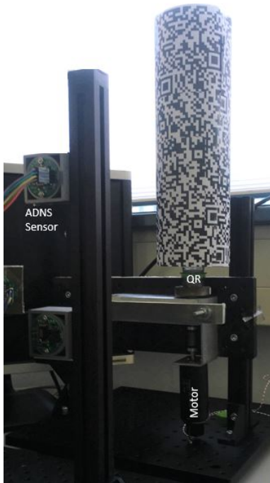
Fig. 18: Simple analog setup for Optic flow detection
