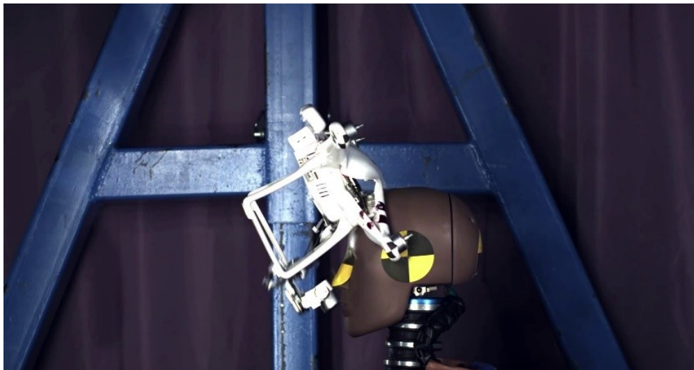
Figure 1-2: Indoor-scenario drone crash indicating potential damage to humans [2]
