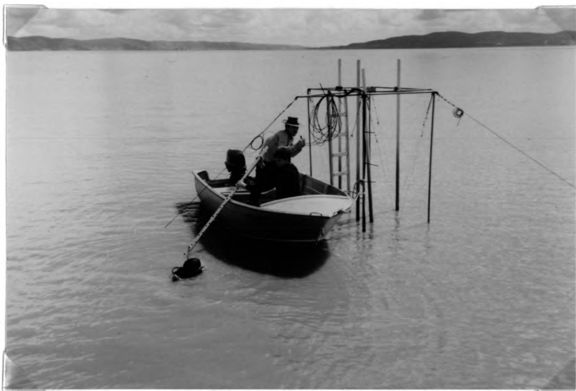
Figure 5.8 Installing the Zwarts poles of the array
