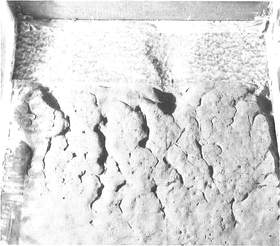
Fig. 102. Channel formation in the sand surface (geotextile and granular filter removed).
