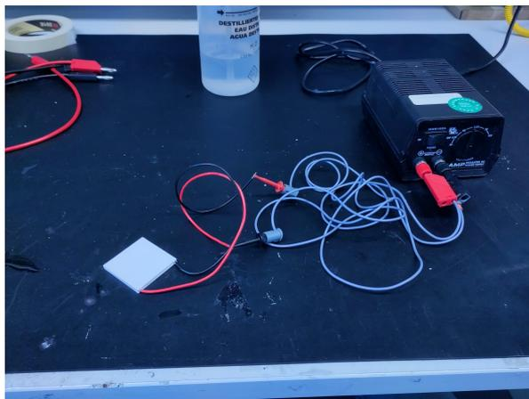
Figure 4.3: 2 amperes regulated DC power supply connected to a Peltier module.
