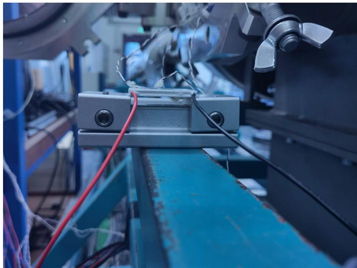
**Figure E.1:** Set up to measure the temperatures on the hot and cold side of the TEC1-12706 Peltier module.
