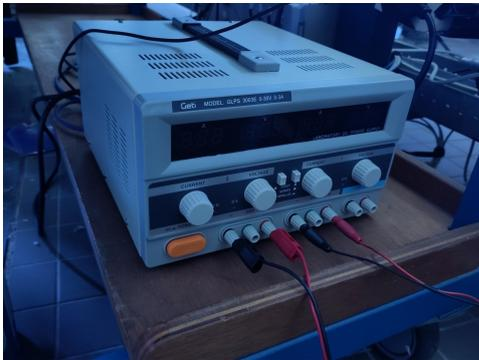
**Figure E.7:** GLPS 3003E 0-30V 0-3A power supply
