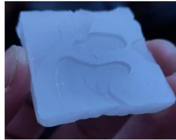
**Figure 4.9:** Bubbles in paraffin after phase change test.
