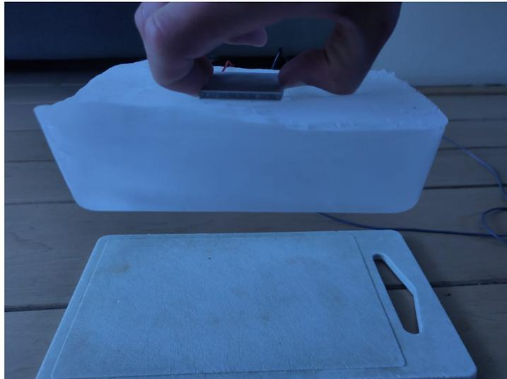
**Figure 6.1:** Experiment 1 - Proof working mechanism of ice adhesion with Peltier module.
