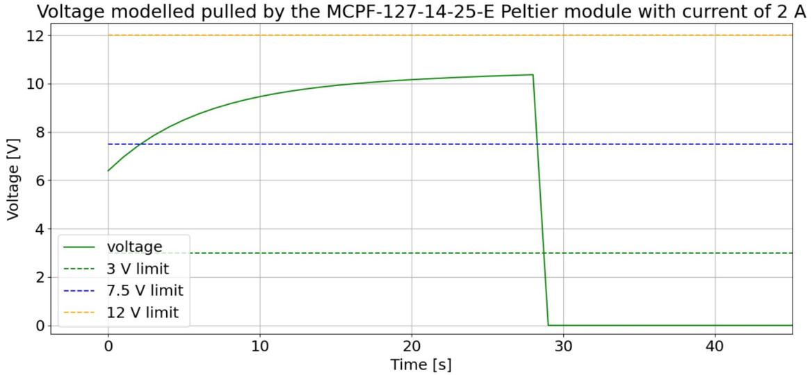
**Figure C.3:** Modelled voltage of MCPF-127-14-25-E module for a current of 2 A.
