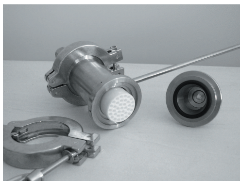
Figure 3.1: Multi-channel monolithic high-silica MFI type zeolite membrane and module.
