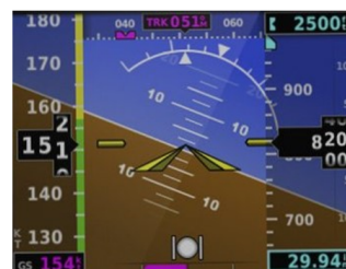
Figure 1. Horizon Errors in which the horizon symbol on the AI (left) is mistaken for the bank angle of the aircraft from a rear view (right)
