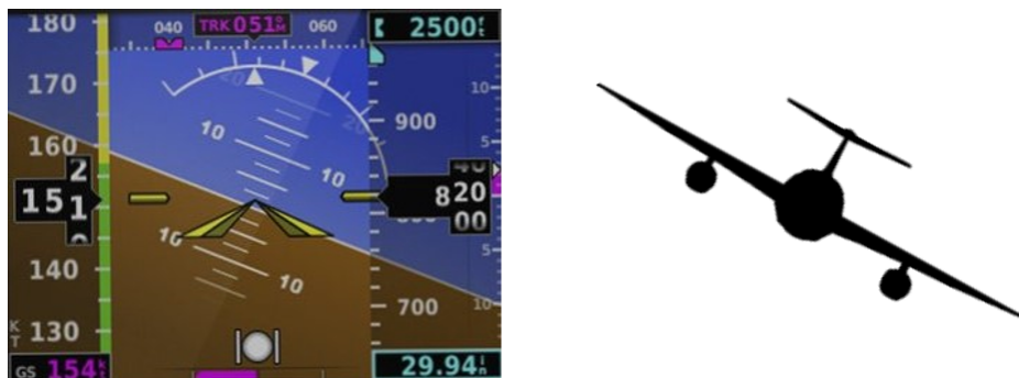
Figure 2.6: Horizon Errors in which the horizon symbol on the AI (left) is mistaken for the bank angle of the aircraft from a rear view (right)
